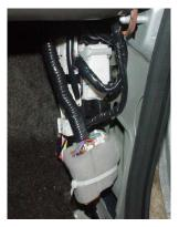
Without AMP: Secure to lower bracket opening.
